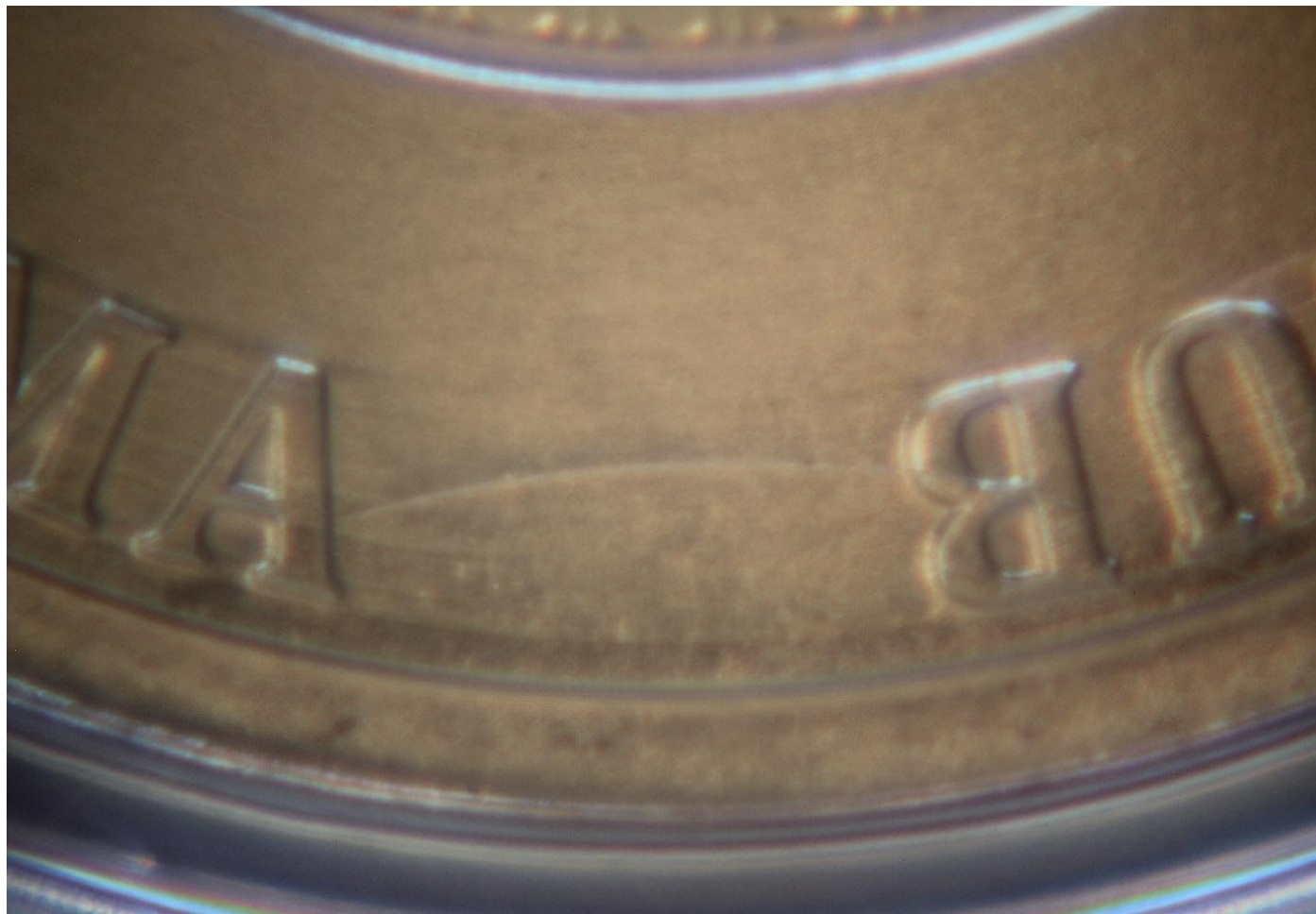
Figure 9 Nickel Medal with Die Crack, Enlarged
